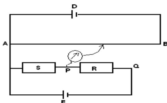
In the circuit shown above D is a driver cell of negligible internal resistance and e.m.f. 3V. AB is a uniform slide wire of resistance  $20\Omega$ . S is a standard resistor of  $5\Omega$ . E is a cell of e.m.f. 2.5V. R is an unknown resistor. When the galvanometer is connected at P the
