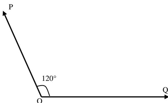
The force P has a magnitude 20N and Q has a magnitude of X newtons. The resultant of P and Q is 3X newtons. Find;
